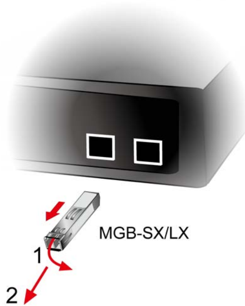
Figure 2-1-8 How to Pull Out the SFP Transceiver
