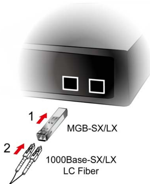
Figure 2-1-7 Plug in the SFP transceiver
